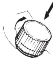
\* When locking the crown, turn it slowly with care, ensuring that the screw is properly engaged. Be careful not to forcibly push it in, as doing so may damage the screw hole in the case.
