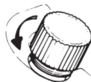
[How to lock the screw lock type crown]
